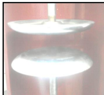
Fig. 5. Two parallel electrodes system without any particle contamination.
