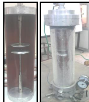
Fig. 1. Test vessel with electrode system.
